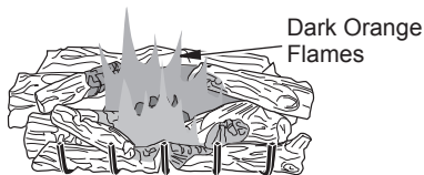
Figure 23 - Incorrect Burner Flame Pattern
